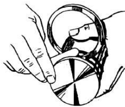
Fig. 2 - Checking Ring Side Clearance
