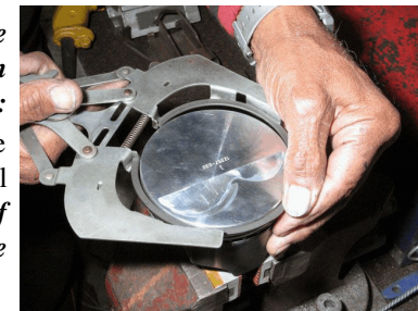
Fig. 3 - Using Ring Expander
